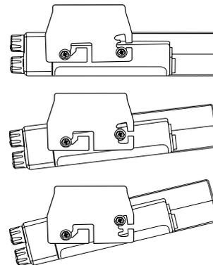
3. To remove the transceiver, unscrew all fixing hardware, and hold the transceiver in the way that it won't fall from bracket.
