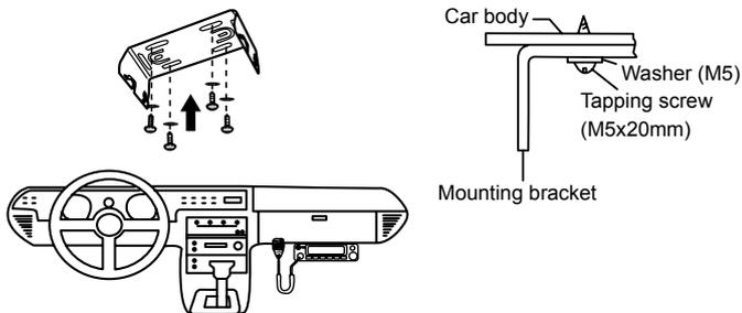
2. Position the transceiver, then insert and tighten the supplied hexagon SEMS screws.
