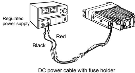
2. Connect the transceiver's DC power connector to the connector on the DC power cable.
