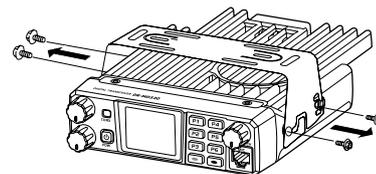
4. Install mic hanger unit. Install the mic hanger in the vehicle using the supplied self tapping screws (2pcs) and washers (2pcs).
