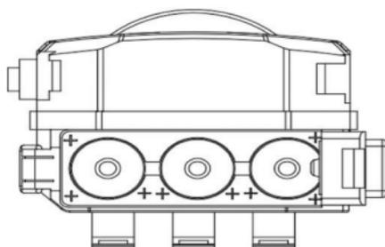
Remove the protective cover located on the side of the camera and insert a micro SD card and a SIM card into the dedicated slots.
