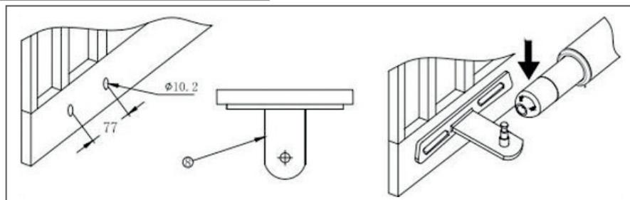
1. Drill in the gate 2 holes of 10.2 mm each to a distance of 68 mm one from each other.
