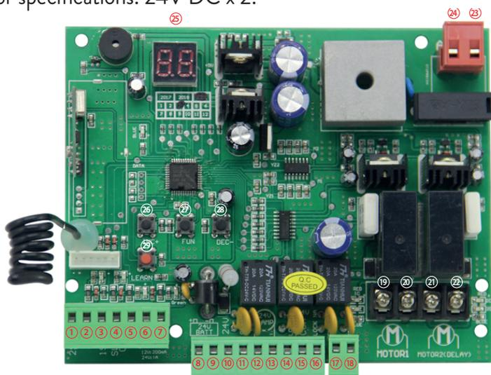
1. 2SIDE+COM: for connecting any external device that controls double gates (non-energized relay)
