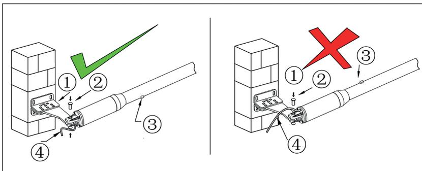
**Left image:** the power cord and the drain hole are correctly positioned.
