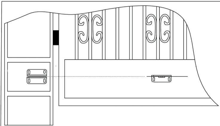
Make sure that the height of installation of the rear bracket is equal to the height of installation of the front bracket. Performing an assembly based on inaccurate measurements can lead to problems in the operation of the piston arm. Also, the opening and closing force will be reduced. Large differences in height between the two brackets can even burn the motor and the piston arm.
