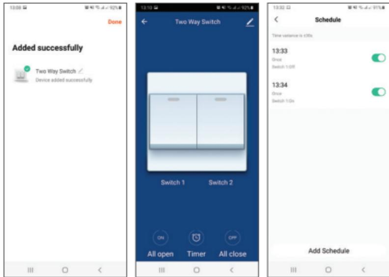
From your Tuya app, you can turn the lights on and off, you can set an hour for the lights to turn on and off automatically, and you can share the smart switch with other family members.
