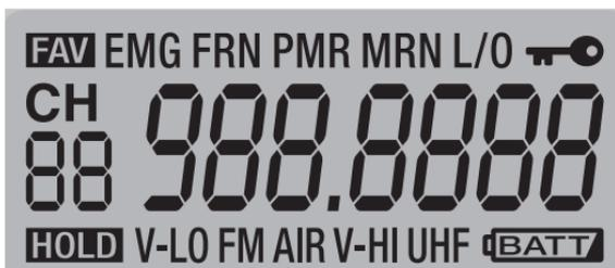
The display has indicators that show the scanner's current operating status. The display information helps you understand how your scanner operates.
