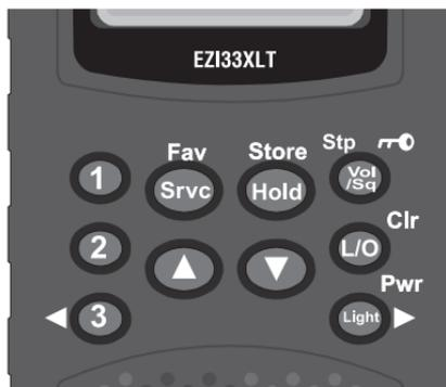
Your scanner's keys have various functions labelled on the key tops and below the keys.
