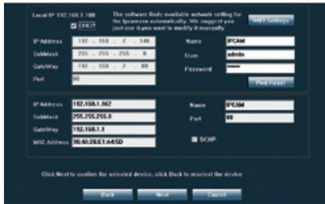
6. Open **Internet Explorer** and input in the address bar **your camera's IP** or return to the list of cameras in the application **Serach Tool** and double-click on the camera you want to view. It will open automatically **Internet Explorer**.
