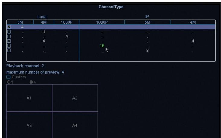
You can simultaneously connect the following types of cameras to this DVR:
