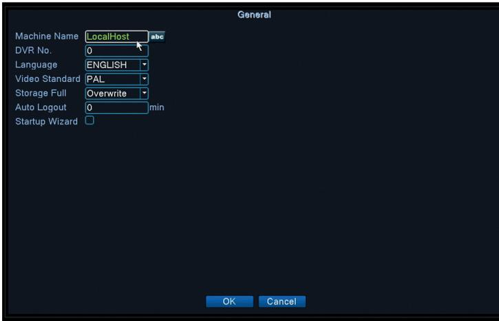
Set the system name, display language, behavior in case of full HDD (overwrite or stop recording), automatic logout period, or enable quick setup guide display each time the system is restarted.
