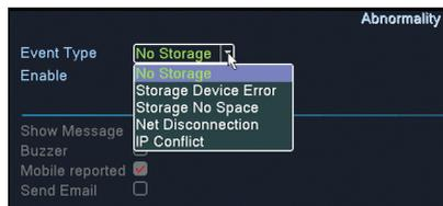
Activate the alert function in case of missing image or signal and set the behavior in case of alert: display alert message on the screen, upload via FTP, send email or notification on the mobile phone.
