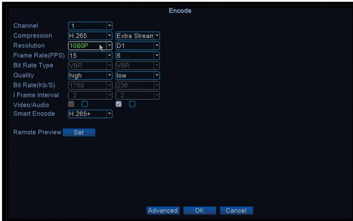
Set different video parameters such as compression, resolution, frames per second (FPS) or quality for each channel.
