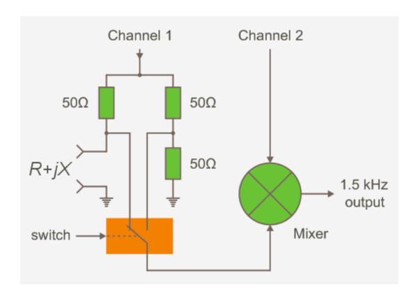
The switch which is controlled by the CPU feeds the signal from the certain side of the bridge to the mixer chip. When the load is totally active and its resistance is  $50 \Omega$ , the bridge is balanced and the switch outputs the same signal in both positions. This eliminates the need of calibration of the analyzer, also giving very good precision near SWR=1.
