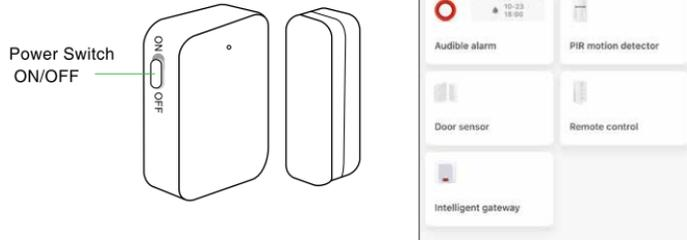
**Adding remote controller:** Switch it ON, the alarm indicator flashes 3 times and stop means coding successfully.
