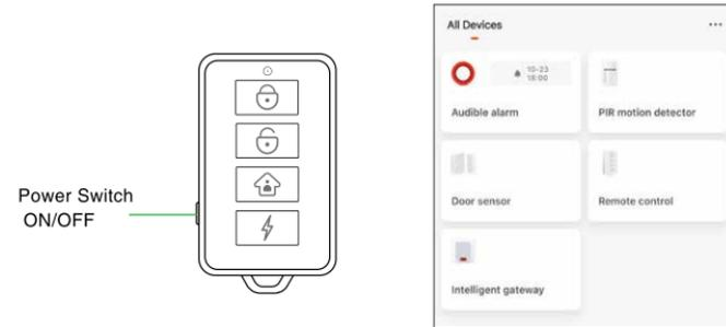
**Adding wireless siren:** Switch it ON, 1 Dee sound, and alarm indicator flashes 3 times and stop means coding successfully.
