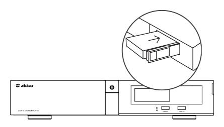
**Note:** Do not load or change the hard disk while the power is on to avoid that the device or the data of hard disk be damaged. If it is a brand-new hard disk, please format it before loading it to the device. This device support following formats of hard disk: EXT3, EXT4, NTFS, FAT32, EXFAT.
