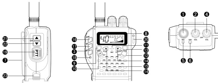
**1. Antenna connection:** fix a compatible antenna (not included in the package). To get better performance, you can use an external antenna that plugs into the included adapter.
