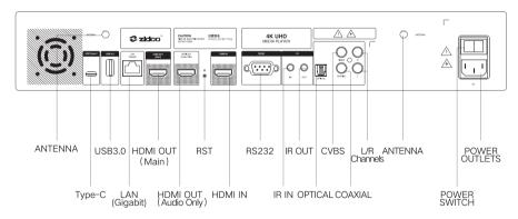
Instruction to installation of the antenna: Please insert the two antennas in the parcel into the antenna ports in the above diagram.
