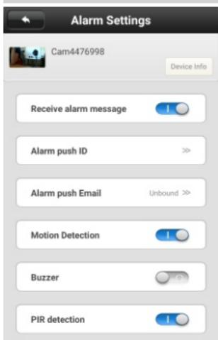
To use the motion detection function you need to make sure the system is armed (the lock bellow the image is closed, press on it to close it) then enable the alarm settings like in the picture.
