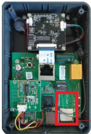
The outdoor unit support local recording of images on a micro SD memory card that you can buy separately. We recommend using class 4 or higher max 64GB memory card.
