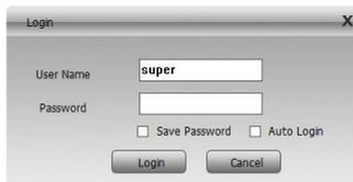
*Note: You can disable the password request when you exit the account by going to System - Local config - Base config. Uncheck "Password is required before exiting".*
