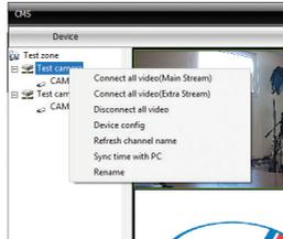
**Connect all video (Main Stream):** conecteaza toate camerele cu flux principal
