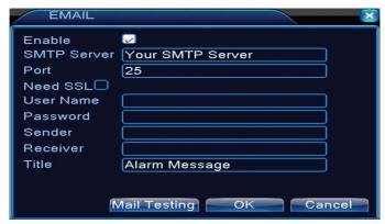
If the alarm is on or the connections are made, the system will send an email with alarm information and photos to the set address.
