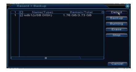
**Detect:** detects the USB recording drive connected to the NVR
