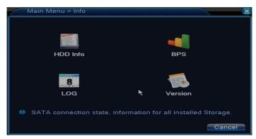
The interface provides detailed information about the storage device, BPS (displays the Kb / s transfer stream and the capacity of the MB / h storage device in real time), event history, and software version.
