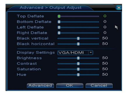
The same interface can be accessed by entering the Main menu - Advanced - Output adjust
