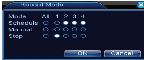
Shortage to set recording mode on each channel. More detailed recording settings can be made by accessing the Main Menu (Main Menu) - Main menu (Recordings) - Record conf (Record Configuration).
