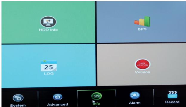
The interface provides detailed information about the storage device, BPS (displays the Kb / s transfer stream and the MB / h storage capacity in real time), event history, and software version.
