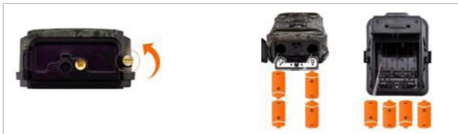
**Step 3: Insert SIM card (3G Model Only) and SD card**
