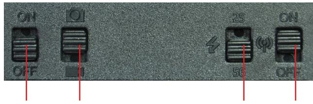
Power switch      Camera/Video switch      IR LEDs Group switch      GPRS switch
