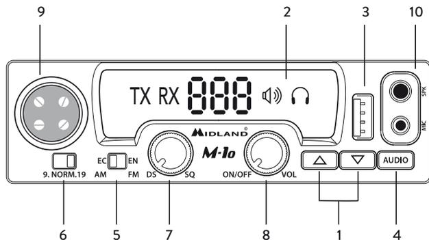
1. **UP/DOWN buttons:** channel selection. Short press: increase/decrease of the channel number; long press: quick scroll of the channels.
