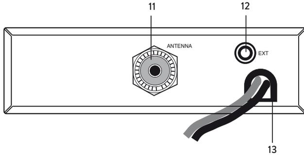
11. **Antenna connector:** PL connector type.
