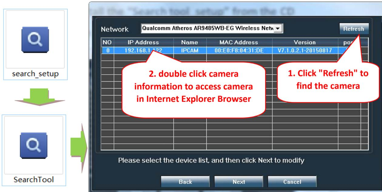
Click "Next" and you can modify network parameters of the camera, according to your network settings. You can use DHCP setting for faster configuration .
