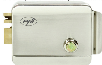
Yala electromagnetica PNI H1085A Fail Secure comanda de tip NO / Normal Deschis / impuls 12V 0.5 secunde
