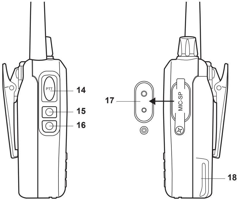
14. **PTT:** push it to transmit (led lights red) and release it to receive (green led).
