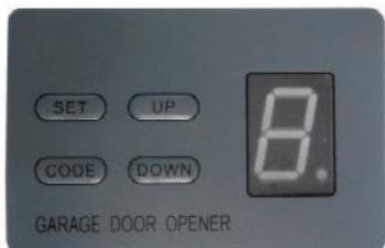
Long press the “SET” button until the LED screen displays the number 1.
