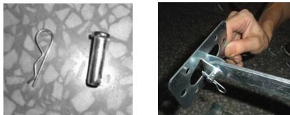
Attach the L-shaped arm to the handle on the toothed belt drive and secure it with the locking pin..
