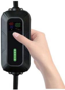
Press the touch button on the portable charging station for 3 seconds. The power indicator will blink. Briefly press the touch button to set the charging current and time.
