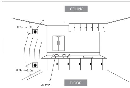
3. Fasten the screws firmly into the wall, then hang the gas detector.
